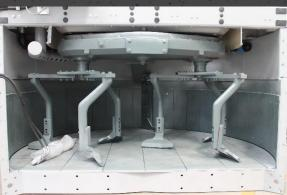
**Planetary PW**, have been specially studied for the production of concrete for the use in the precast industry, the Witech planetary mixers main features are, perfect and smooth mixture in the shortest time, high productivity at constant mixing quality, long-lasting use at low operational costs.
