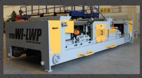
Witech LWP light wall clay panel machine, casting machine for manufacturing of non-load bearing, precast partition wall panels.
