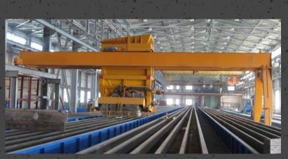
WiTech has specialized in the production of automatic and manual plants for the production of foundation POLES. It is equipped with an automatic system for distribution of the concrete in the formworks which are provided with heating system and automatic vibration.
