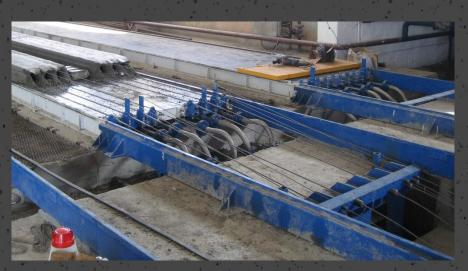
The exit bridges are needed to use the full length of the casting beds during the production. The exit bridges are special metal bridges for the correct exit of the machines at the end of the casting bed.
