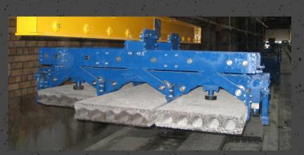
Witech Lifting beam for concrete elements complete with automatic clamps for the Hollow Core Slab slabs and for Light Wall Panels
