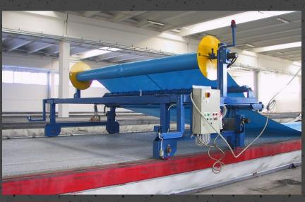
Witech CARRIER for Plastic Covering This machine unwinds and winds the cover sheets on the elements travelling on casting beds rails.
