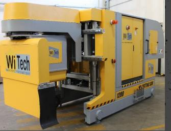
The Witech cutting machine is designed for making the most used types of cuts of the pre-stressed hollow-core slabs, and other elements with max height 500 mm,
