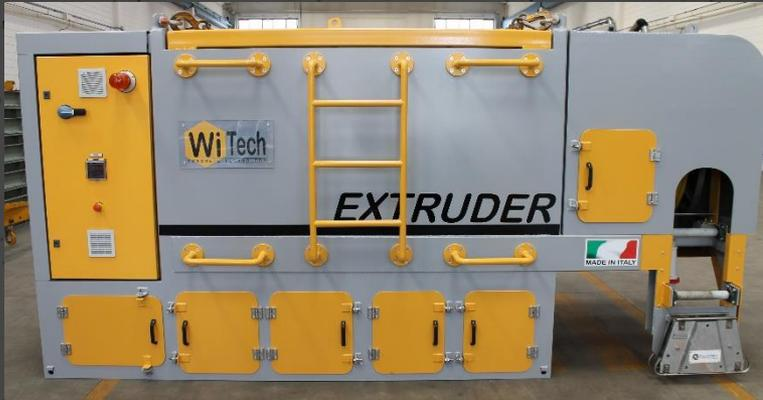
The machine is composed of two groups, a control and concrete feeding unit, called Silo, and a mechanical part dedicated to the proper hollow-core slab production, called Assembly.
