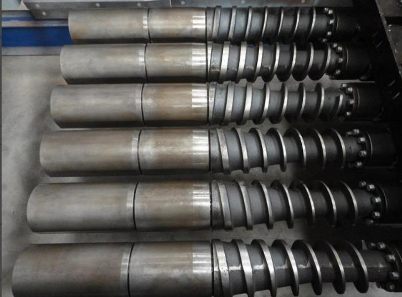
The Witech Extruder is made with a new technology, the machine doesn't use any internal vibrators for concrete compaction,
